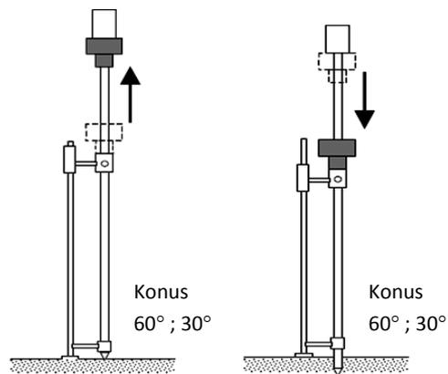
Gambar 5 Cara Kerja Penetrometer Konus Dinamis (DCP) (Dynamic Cone Penetration Test (DCPT) for Subgrade Assessment, 2003)
