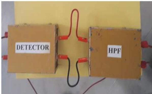
Gambar 13. Pendeteksi Partial Discharge
