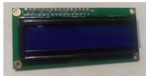
Gambar 5. LCD 16 x 2 with I2C ( Depan )
