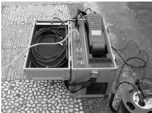
Gambar 1. Ecoline 6000 Gas Analyzer
