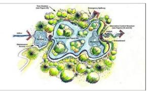
Figure 5: Typical constructed wetland system Source: Virginia DEQ Stormwater Design Specification No. 13
