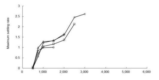
Fig. 4. Maximum Settling Rate vs Water Content
