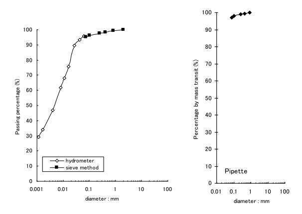
Fig. 2. Grain Size Distribution Curves
