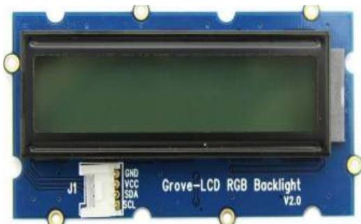
Gambar 5. LCD Display 16x2
