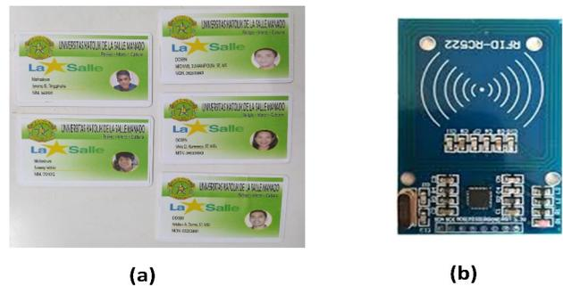
Gambar 6. (a) Kartu (RFID tag) ; (b) MFRC522 (RFID reader)
