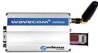
Gambar 2. Modem GSM
