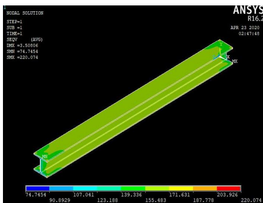
Gambar 16. von-Mises-stress (Ruang Arsip E)
