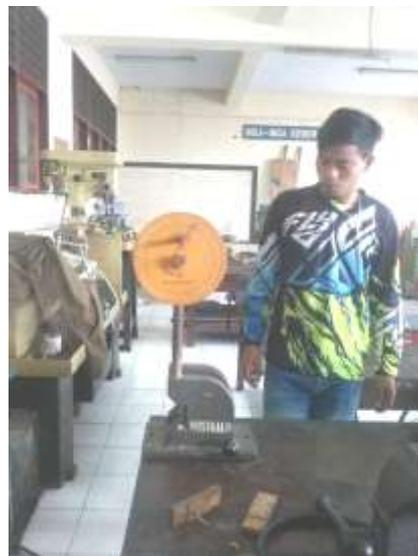
Gambar 5.3 Alat Uji Impact Mobile
