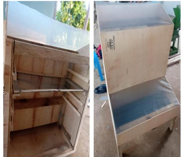
Gambar 3. Rak pengering *Low Cost Modular Solar Dryer*
