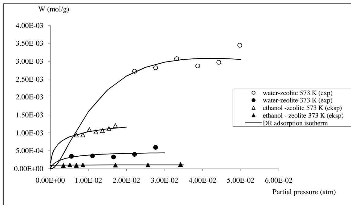
**Figure 1.** Adsorption isotherm of water and ethanol on zeolite A
