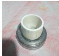
Gambar 5. *Bearing* Yang Dipasang Pipa  $\frac{1}{2}$  Inchi
