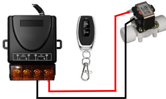
Gambar 1. Rangkaian antara Relay Switch Remote Control dan Electric Solenoid Water Valve
