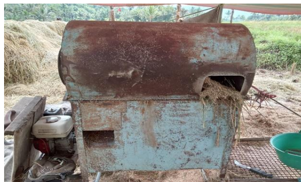
Gambar 1. Alat Perontok Padi Drum Silinder Tertutup Tipe TH6-G88
