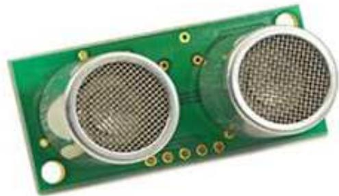
Gambar 8. Sensor Jarak SRF04
