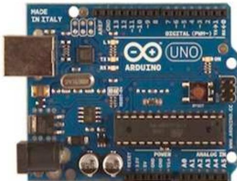
Gambar 5. Board Arduino Uno
