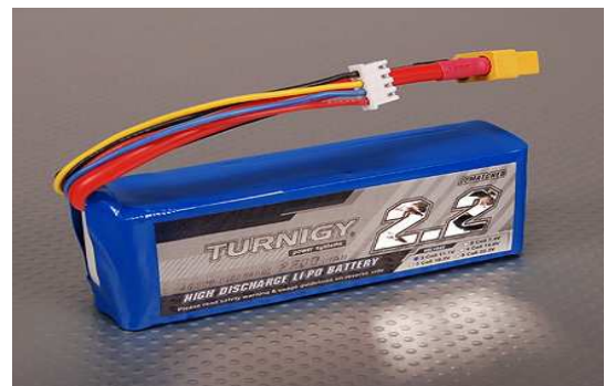
Gambar 6. Battery Jenis Turnigy 2200 mAh 11.1 V
