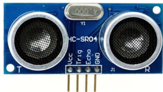
Gambar 2. Sensor Ultrasonik HC-SR04
