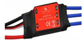
Gambar 6. Electronic Speed Controller (ESC)
