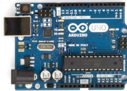
Gambar 3. Arduino Uno ATmega328 [1]
