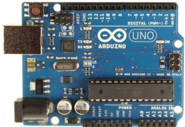
Gambar 2 Contoh Papan Arduino UNO R3
