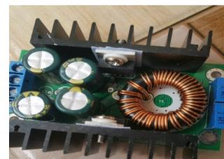
Gambar 7. Modul Buck Step Down Converter
