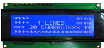
Gambar 2. LCD (Liquid Chrystal Display) 20x4 Karakter
