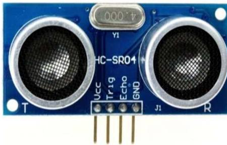
Gambar 7. Sensor Ultrasonik
