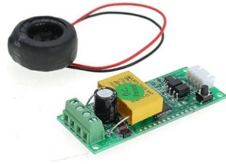
Gambar 1. Sensor Arus PZEM-004t[12]
