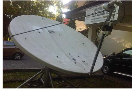
Gambar 10. Antena VSAT 1.8m
