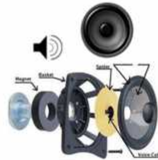
Gambar 5. Simbol Umum dan bagian-bagian Speaker
