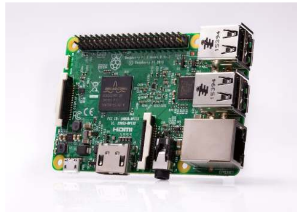
Gambar 2. Raspberry Pi 3 Model B
