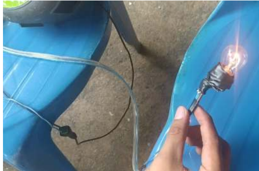
Gambar 15 Dokumentasi bohlam DC 24V, 21W
