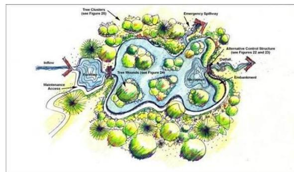
**Figure 5: Typical constructed wetland system**
