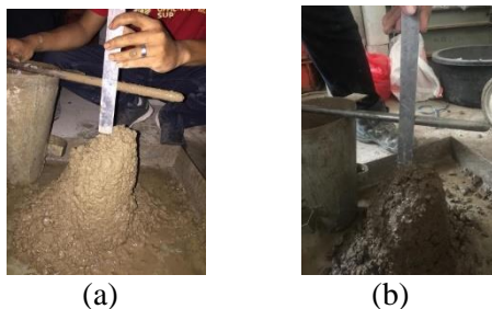
Gambar 6. (a) Slump Geser, (b) Slump Runtuh
