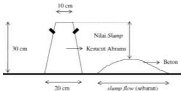
Gambar 1. Sketsa *Modified Slump Test*
