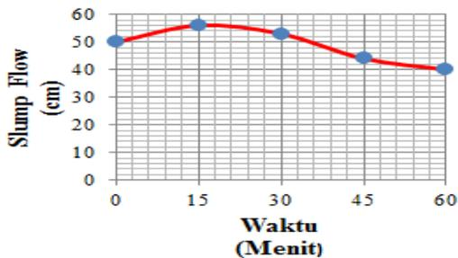
Gambar 13. Hubungan Slump Flow Terhadap Waktu (Superplasticizer 2%)
