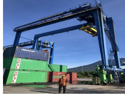
Gambar 2.1 Rubber Tyred Gantry
