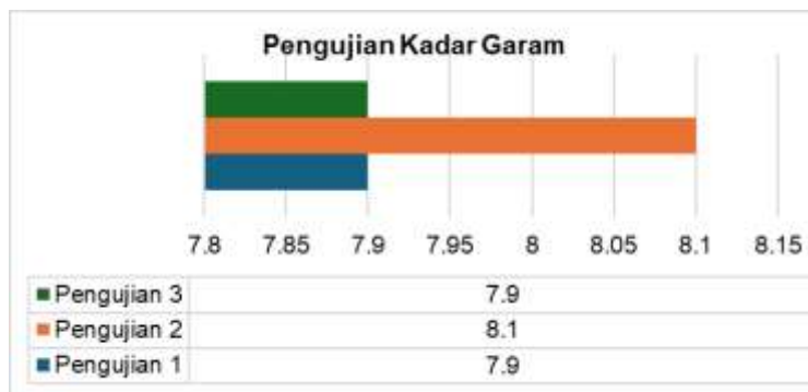
Figure 3. Graph of NaCl content in salt from a tunnel-based salt house based on three tests
