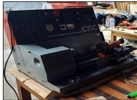
Gambar 1.1 EMCO Compact 5-PC CNC Lathe di Jurusan Teknik Mesin Unsrat
