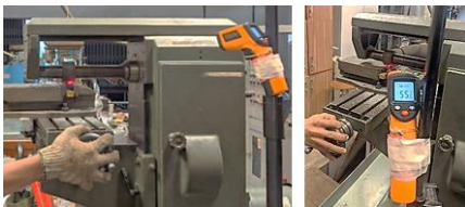
Gambar 3.7 Proses Pengukuran Temperatur Geram
