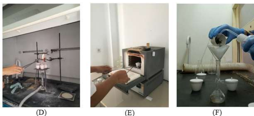
Figure 4. Combustion using a Bunsen burner (D), ashing in a furnace (E), filtration using Whatman No. 42 filter paper (F), filtration using Whatman No. 42 filter paper
