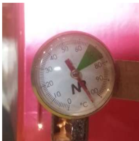
Figure 4. Photo of analog thermometer indicating chamber temperature above 100 °C during operation at 150 W.
