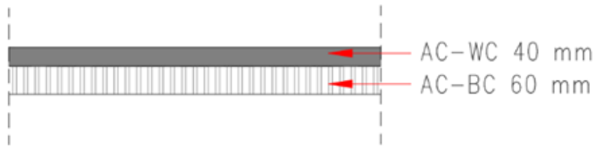
Gambar 5. Tipikal Penanganan Rehabilitasi Mayor
