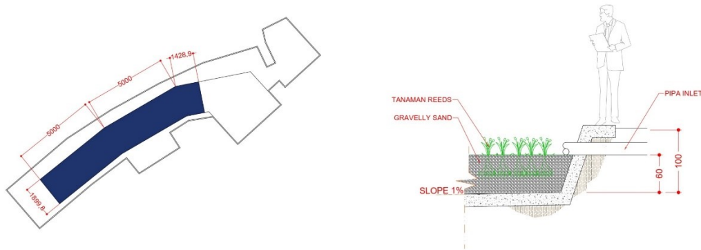
Gambar 3. Dimensi dan Detail Constructed Wetland
