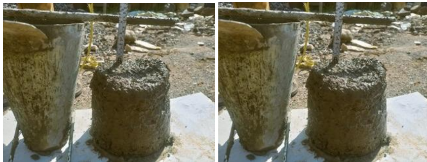
Gambar 7. Slump Test Atap Dak
