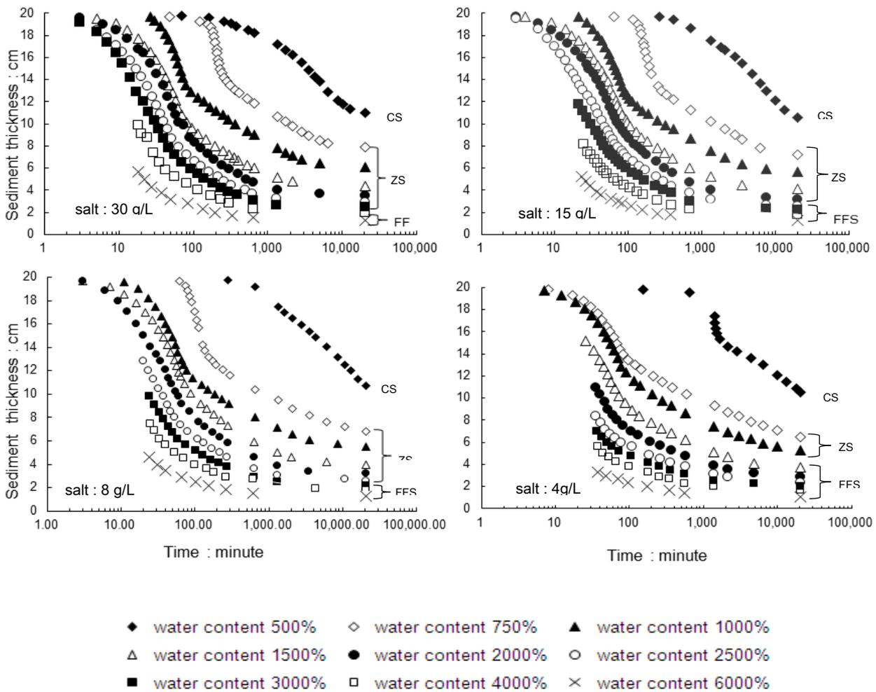
Fig. 3. Sediment Thicknes vs. Time according to Settling Types
