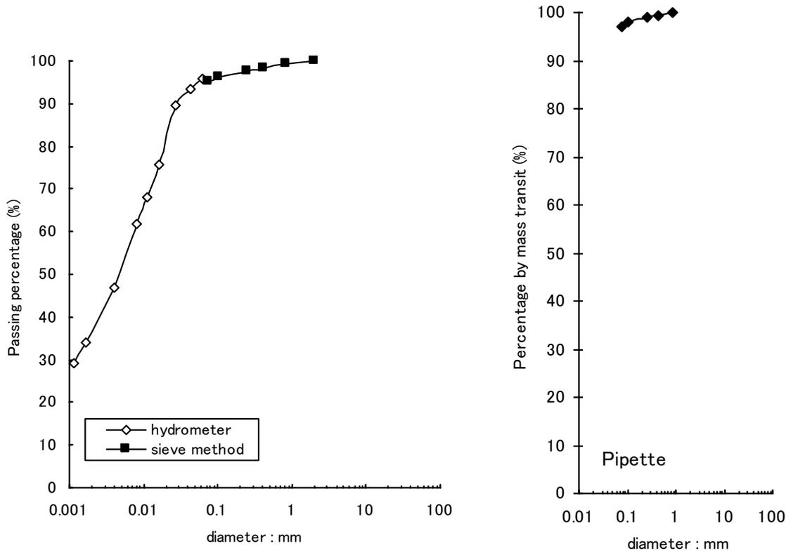
Fig. 2. Grain Size Distribution Curves
