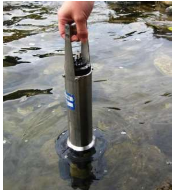
Figure 1. Measurement using CTD meter
