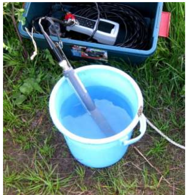
Figure 2. Measurement using multi item water quality meter
